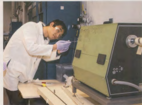
Xiaotian Zhang, an undergraduate student in materials science and engineering, removed a sample of silicon diselenide from an annealing furnace. The researchers are investigating the use of semiconductor crystalline silicon diselenide ( \text{SiSe}_2 ) as a thin film to sit atop a more conventional silicon solar cell. They are exploring how best to synthesize the material into a thin film as well as how to treat or "dope" it with other elements to improve its photovoltaic qualities.
