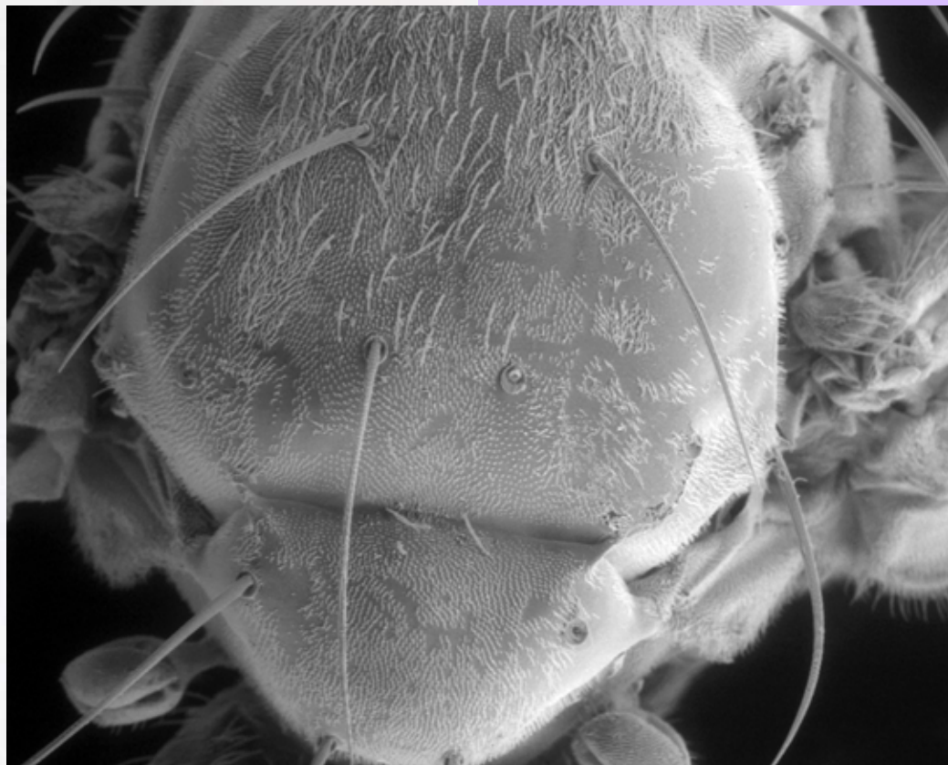
Below: The head of a fly coated with chalcogenide glass is magnified at 150x.
