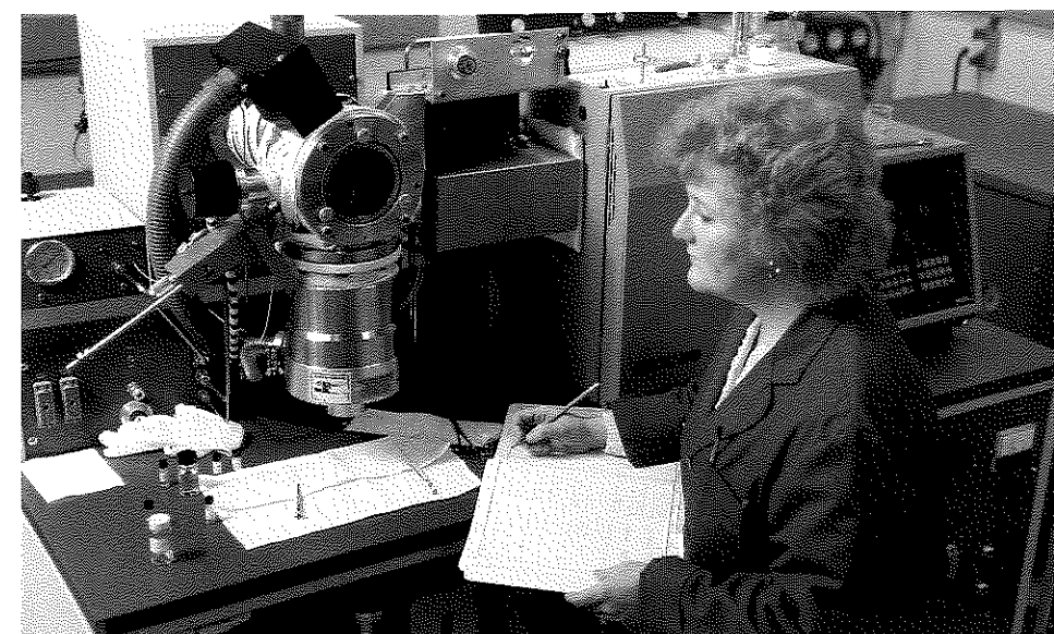
A fuel science student analyzing synthetic liquid fuel using a gas chromatograph/mass spectrometer.
