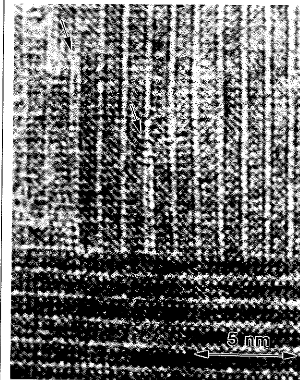
Figure 1. High-resolution TEM micrograph of a grain boundary in \text{YBa}_2\text{Cu}_3\text{O}_{7-x} with a rotation of 90° from one side to the other. The brightest rows of dots represent the Cu-O basal planes of the unit cell and are spaced by 1.17 nm. The geometrical mismatch at the interface results in defects, including additional atomic layers (stacking faults) in the upper grain (arrowed). The faults terminate within 10 nm of the boundary at dislocations, which are aligned parallel to the viewing direction.
