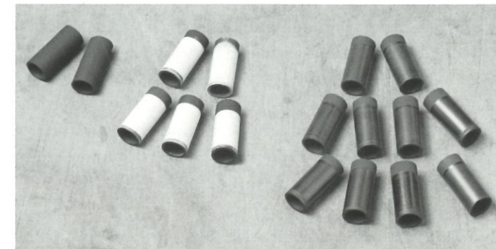
As-received ceramic tube sections (extreme left); tubes with unfired EPD zirconia coating (middle); and sintered tubes with a gas-tight zirconia coating (right). Dimensions: length-50mm, diameter-22mm, thickness-2mm. Tubes supplied by the Siemens-Westinghouse Power Corporation, which is using the same variety to produce gas-tight zirconia films with an expensive, sophisticated electrochemical vapor deposition technique for which Penn State now has a cheaper, faster alternative.
